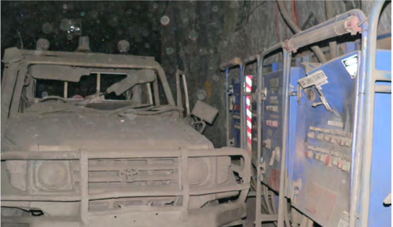
*This photo shows the air blast damage to the shot firer's car, which was 80 metres away from the blast*
